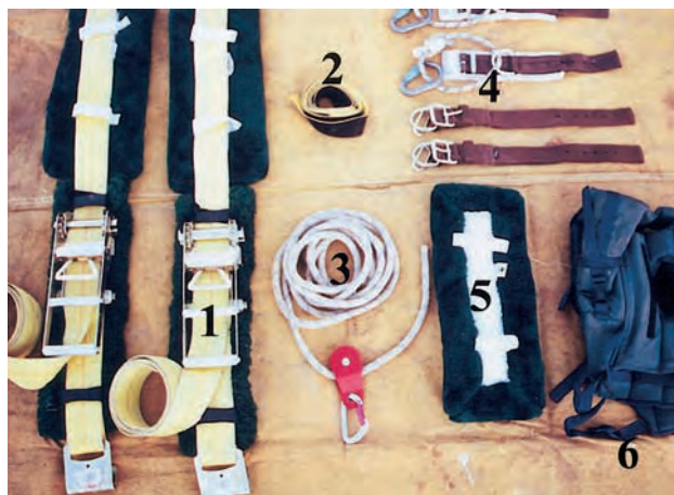
Fig. 8. Accessories for the rescue glide. (1) Three-inch ratchet straps with fleece pads. (2) Webbing with velcro for securing head to glide. (3) Rope, pulley, and carabiner for pulling hobbles. (4) Leg hobbles with Prussik loops and carabiners. (5) Fleece pad protection for rope. (6) Head protection. (7) Ten foot or longer nylon web (not shown).
