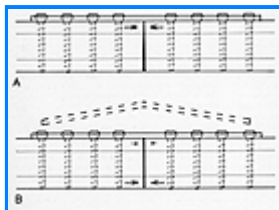
FIG. 16-11 Effects of prebending compression plates. (A) Compression applied to a straight bone using a straight plate will give compression under the plate and a gap opposite the plate. (B) A prebent plate will provide compression on the cortex opposite the plate as well as underneath it.
