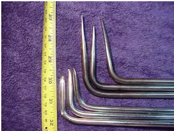
Figure 1: Picks in a variety of angles, lengths, widths, bevels, and points are required for elevating dental attachments. Commercially available picks are pictured at the lower left for comparison.
