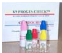
Figure 5. Components of the K9 Proges-Check test kit for measurement of progesterone in canine serum (Endocrine Technologies, Inc., Newark CA). The test is run in clear test wells with three controls. - To view this image in full size go to the IVIS website at www.ivis.org . -
