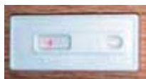
Figure 3. Final result of a test for luteinizing hormone using the Status-LH test kit (Synbiotics, San Diego CA). The pink line is the control, indicating that the test is complete and was run correctly. The absence of a similar pink line beneath the control marker, next to the letter T on the test device, is indicative of a concentration of LH in the test sample of less than 1 ng/ml. - To view this image in full
